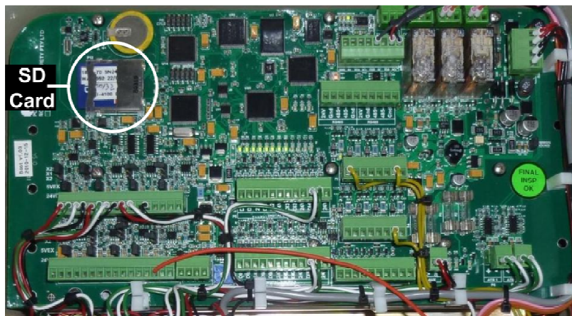
Figure 11 - RCI-4100 Control Unit board showing the SD card
