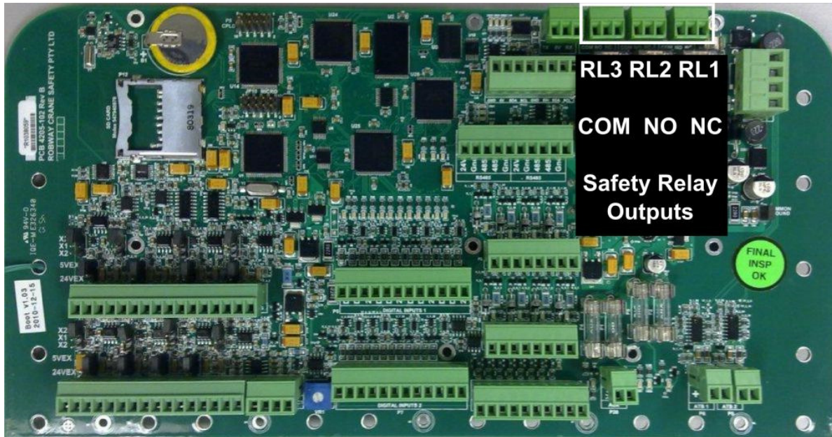
Figure 18 - RCI-4100 Controller PCB showing location of Relay Outputs (RL) Connectors
