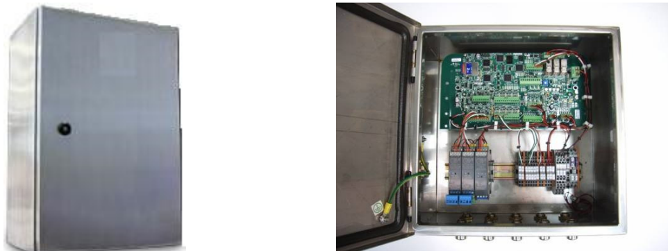
Figure 6 - Typical safe area control unit inside the operator's cabin
