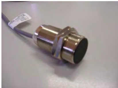
Typical installation of slew/proximity switch
