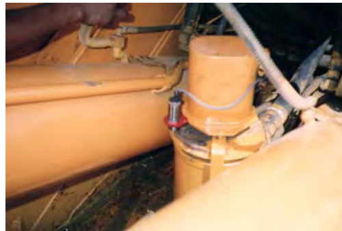
Typical installation of slew/proximity switch
