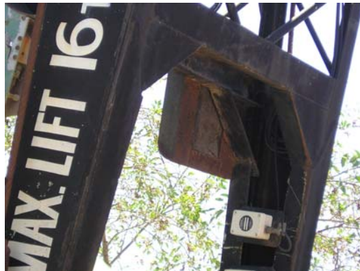
Electronic angle sensor and typical installation at the boom butt section
