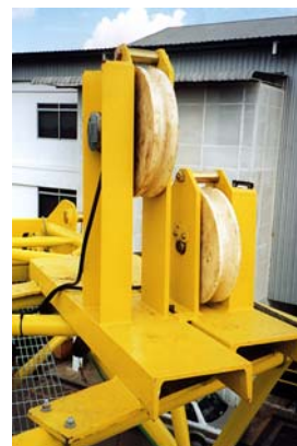
Typical installation of load pins in single sheave dynamometers
