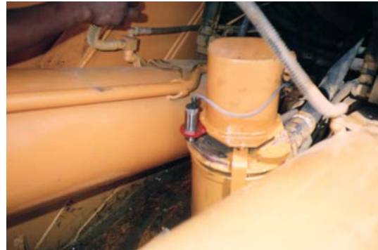
Typical installation of slew/proximity switch
