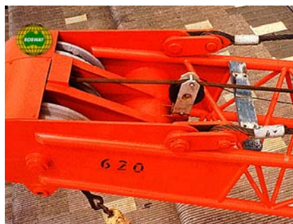
Typical installation of load pins in single sheave dynamometers
