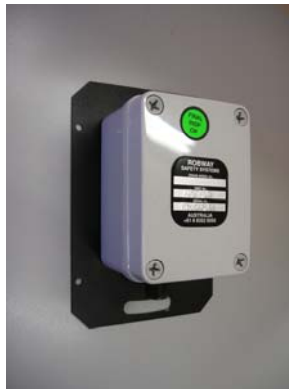
Electronic angle sensor and typical installation at the boom butt section
