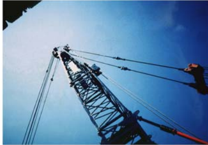
Typical installation of dynamometers/tensiometers on strut boom cranes
