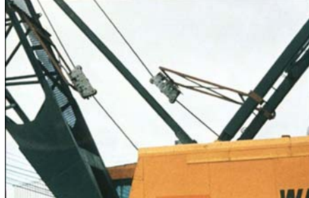
Typical installation of dynamometers/tensiometers on strut boom cranes
