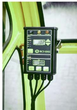
Display unit and typical installation inside the cabin
