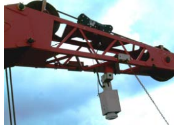
Typical installation of HRT dynamometer
