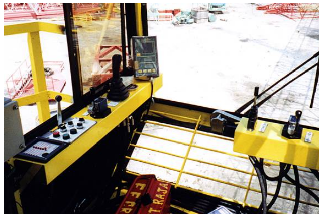
Display unit and typical installation inside the cabin
